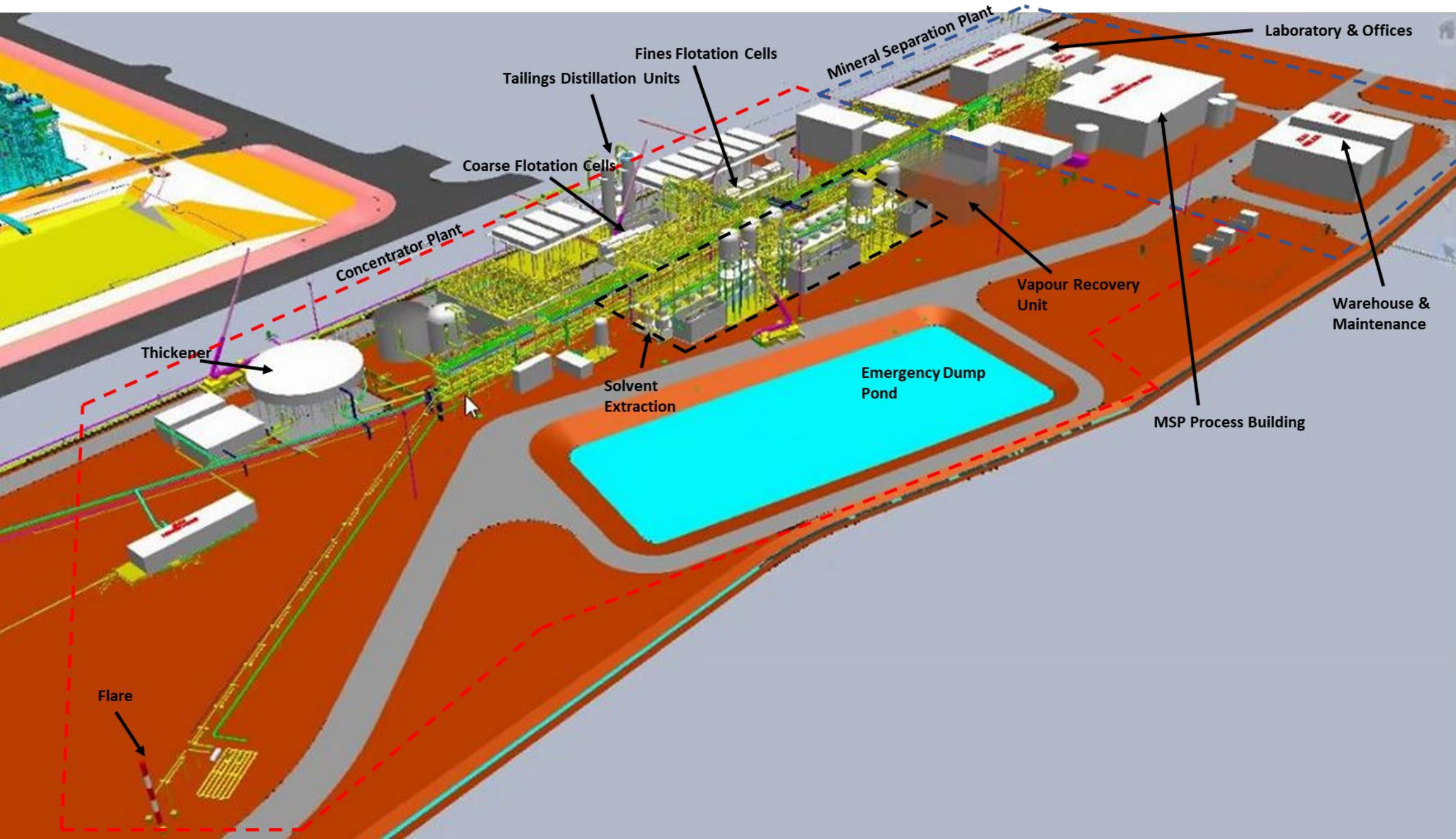
Figure 3. Rendering from the CVW™ optimization study 3D model depicting the plot site.
