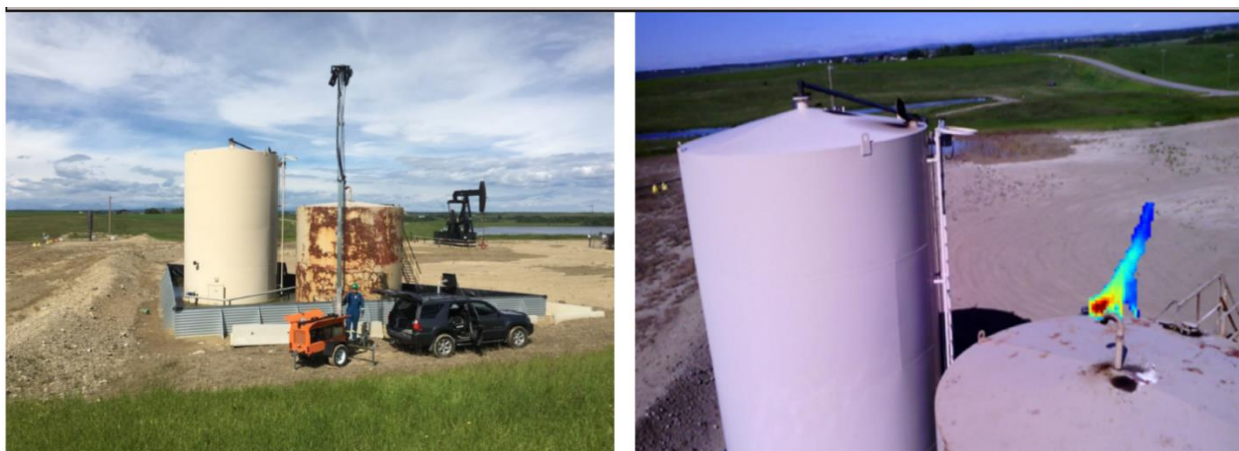
Figure 11 – Installed proof of concept camera(L) and gas detection image (R) from camera at well site near Cochrane, AB
