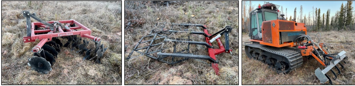
Figure 3. Tow-behind implements tested in this project: line restoration drum, a small acreage disc (left), small acreage harrows (center) and small acreage box blade with tines (right).
