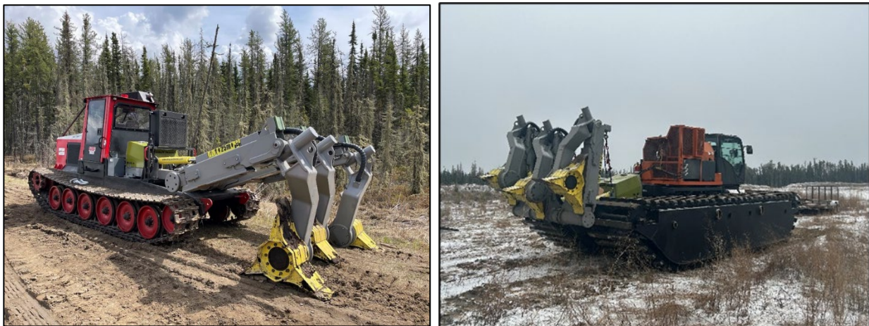
Figure 7. Bracke moulder implements tested in this project: Bracke three-row moulder attached to a KMC prime mover testing in 2022 (left) and Bracke three-row moulder attached to an amphibious pontoon tested in 2023 (right).
