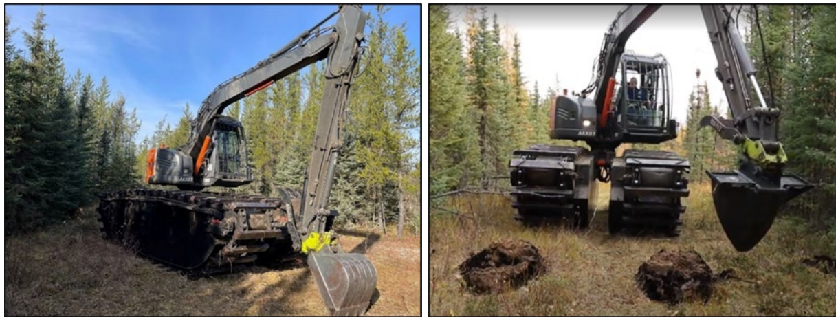
Figure 2. An amphibious prime mover with conventional bucket (left) and a tree scoop modified to work with an excavator quick attach (right).
