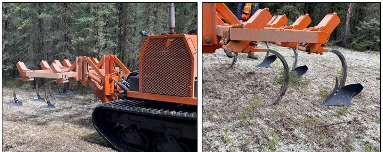
Figure 5. Tow-behind implements tested in this project: cultivator with sweeps (left) and cultivator with potato plow shoes (right).
