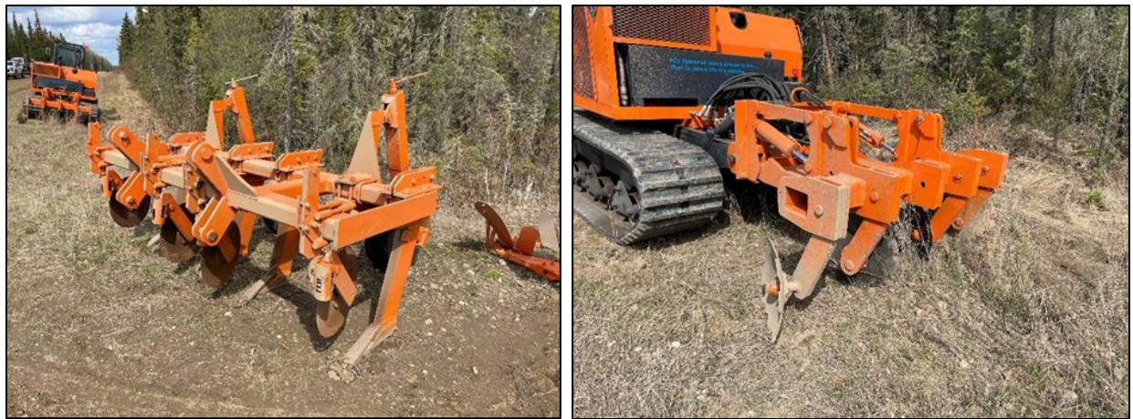
Figure 4. Tow-behind implements tested in this project: ripper shanks (left) and single row disc (right).
