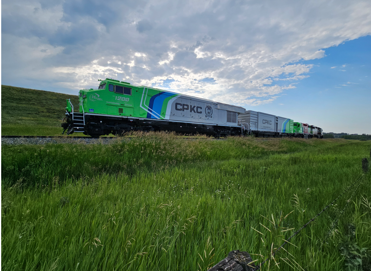
Figure 12 - CP 1200 HHP locomotive and tender during a mainline non-revenue test.
