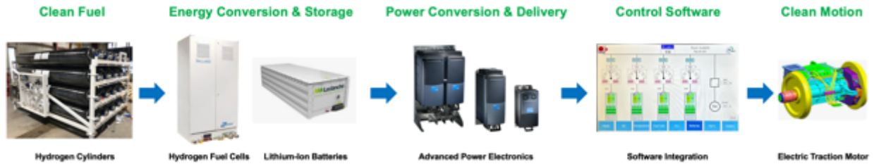
Figure 4 - High-level summary of the process of using hydrogen gas to drive a locomotive electric traction motor and the overall locomotive architecture.
