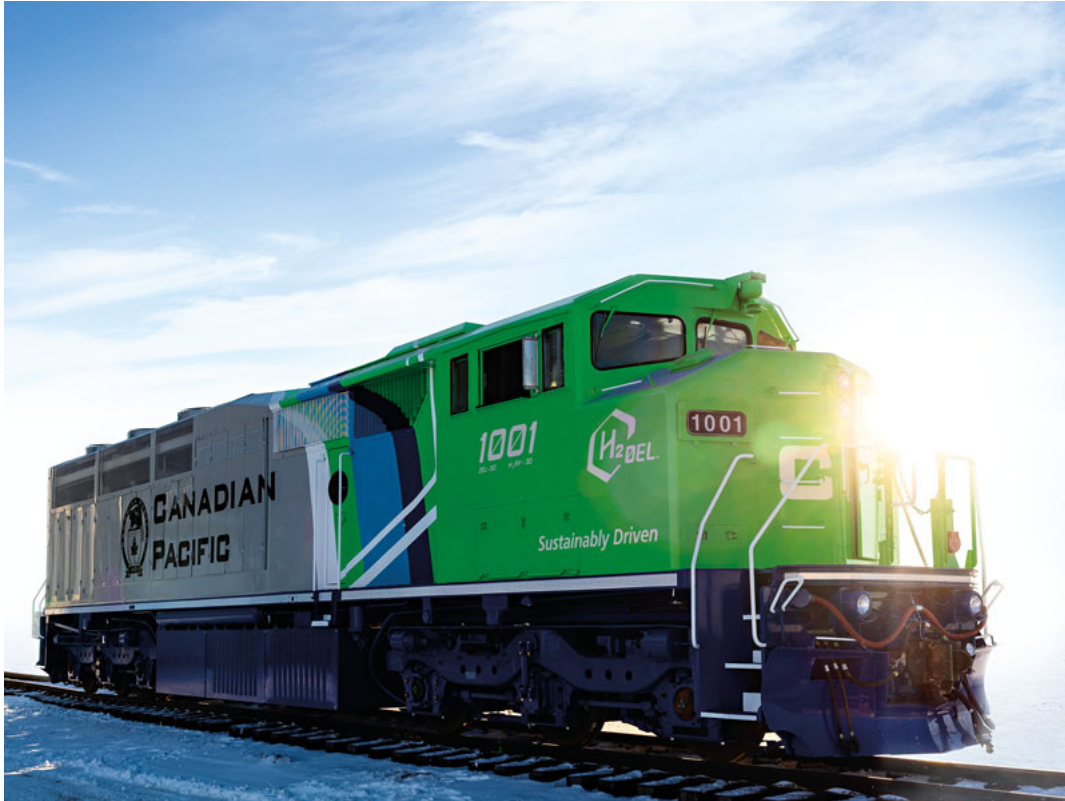
Figure 6 - CP 1001 hydrogen fuel cell battery hybrid locomotive. North America's first for line-haul operation.
