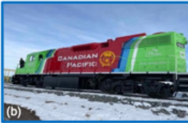
Figure 7 - CPKC's CP1001 and CP1002 Low Horsepower (LHP) locomotives shown in images (a) and (b) and the CP1200 High Horsepower (HHP) locomotive and CP10001 tender shown in (c).
