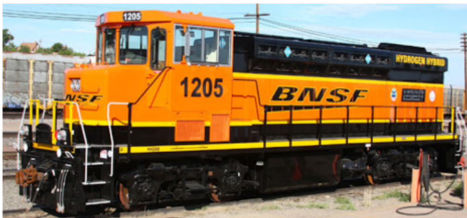
Figure 5 - Hydrogen Hybrid switcher locomotive (Source: RailPicture.net photo Nathan Zachman)
