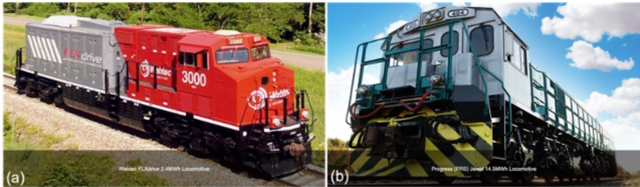
Figure 2 - Mainline designed battery-electric locomotive used within a diesel-electric hybrid consist (a) and terminal switcher battery locomotive (b) from each North American Original Equipment Manufacturers (OEMs) (Sources: Wabtec, Progress Rail).
