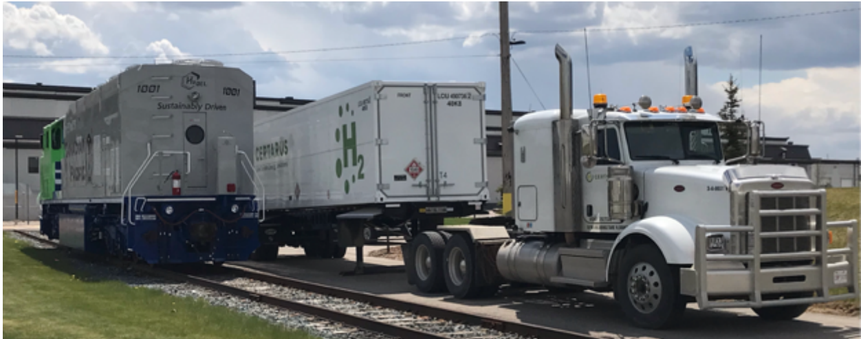
Figure 15 - Certaurus hydrogen gas trailer refueling the CP 1001 via pressure cascade to demonstrate Direct-To-Locomotive ("DTL") refueling.
