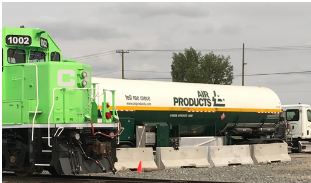
Figure 16 - Air Products liquid hydrogen "Hydra" trailer refueling the CP 1002 to demonstrate Direct-To-Locomotive ("DTL") refueling.
