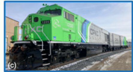
Figure 7 - CPKC's CP1001 and CP1002 Low Horsepower (LHP) locomotives shown in images (a) and (b) and the CP1200 High Horsepower (HHP) locomotive and CP10001 tender shown in (c).
