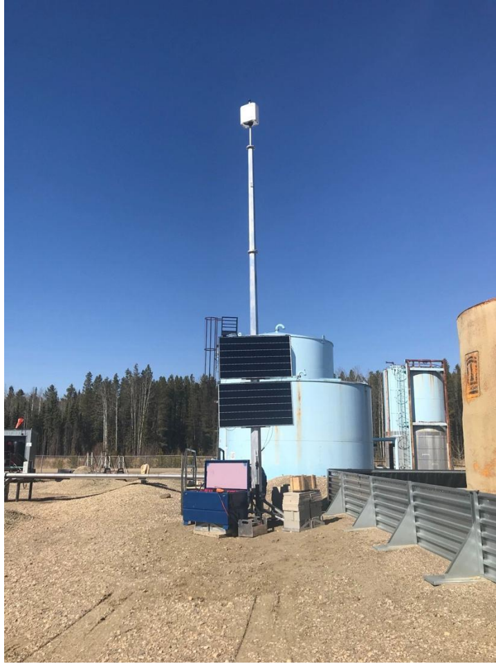
Figure 3-1 Original Kuva Camera with Off the Shelf 9m tower
