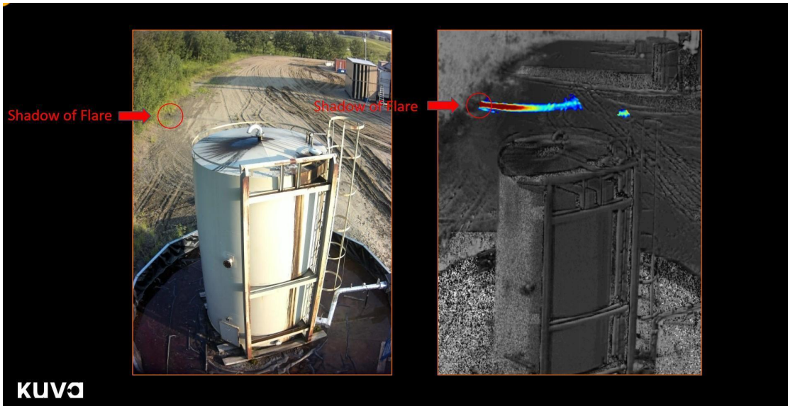
Figure 3-18 Flare Detection at Upstream Site
