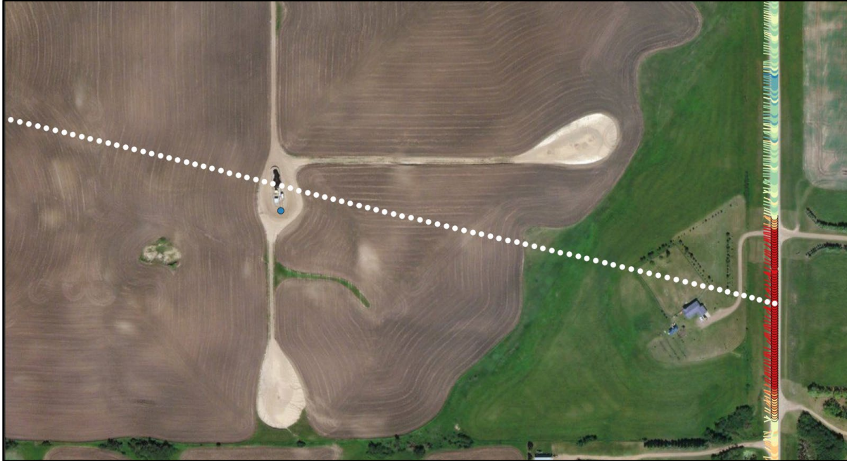
Figure 10: An example of an emissions measurement, attribution and quantification from the Passive modality. In this example, the vehicle path is shown with barbs pointing to the direction of the wind. The red colors indicate higher methane concentration anomalies. This peak was segmented out, and the white dots show the flowtrace (where air was suspected to travel). The attributed site is shown with a blue dot. This estimate was taken passively without the knowledge of the field crews, just as they were driving to another site. The estimated emissions rate was approximately 601 cubic m / day of methane. This site could be prioritized for abatement as this is a relatively large emissions rate from a relatively small site.
