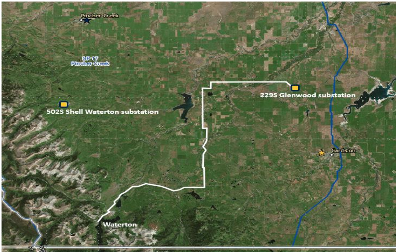
Figure 1: Glenwood Substation 70km radial distribution feeder to Town of Waterton
